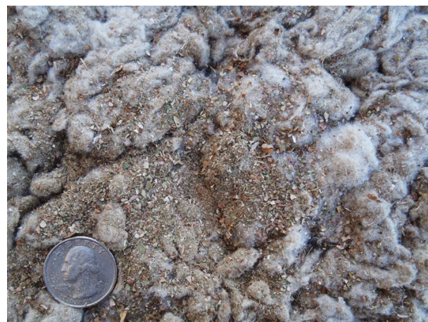
Figure 3. Photograph of typical trash captured by the overflow system cyclones.
