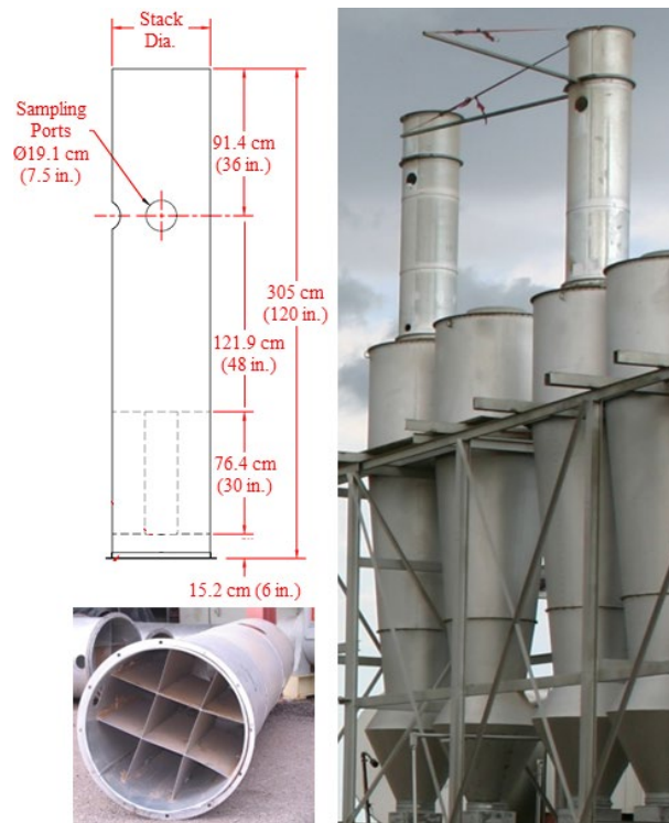
Figure 8. Schematic and photographs of stack extensions with sampling ports and straightening vanes (rail attached to extension above sampling port, at right, supports sampling probe during testing traverse).
