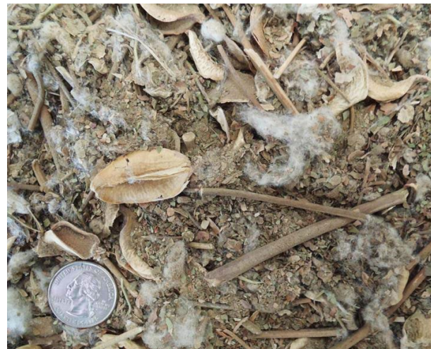
Figure 4. Photograph of typical trash captured by the 1 st stage seed-cotton cleaning system cyclones.
