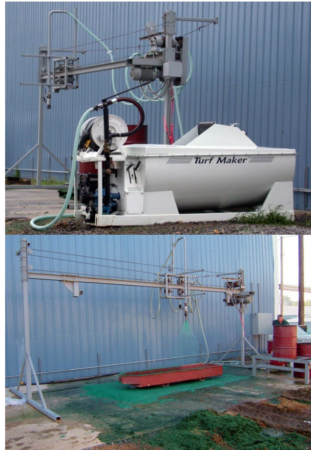
Figure 1. Hydro-mulch application gantry system.
