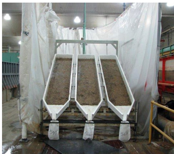
Figure 2. Triplicate soil plot test configuration.
