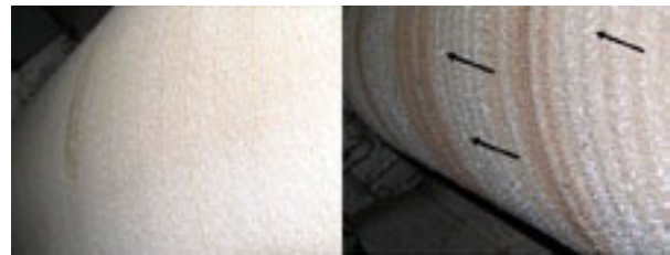
Figure 2. Standard roller covering (left) and experimental roller covering (right) installed in roller gin stands. Note: Fiberglass fibers protruding from experimental roller.
