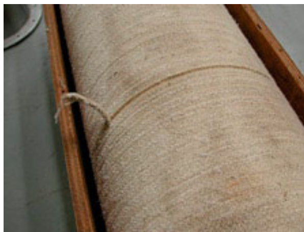
Figure 3. Experimental roller damage after six hours of ginning in a commercial gin plant.
