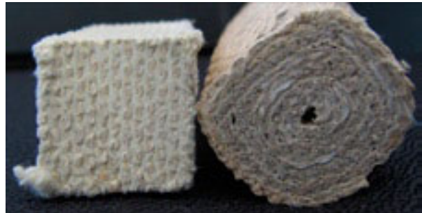
Figure 1. Cross-section of the standard roller covering (left) and the experimental roller covering (right).
