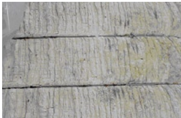
Figure 1. Typical yellow or dark discoloration water damage observed when the polyethylene coverings were removed from the bales in which moisture was added.
