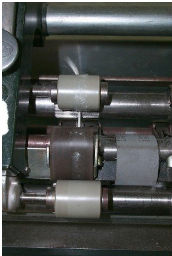
Fig. 4. Sticky deposits on the ring spinning frame.
