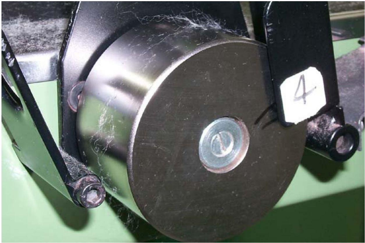
Fig. 2. Sticky deposits on the draw frame creel drive rolls.
