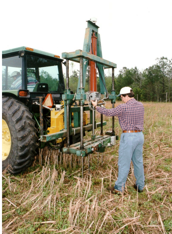
Fig. 2. Multiple-probe soil measurement system that obtains cone index values in five positions across a row.
